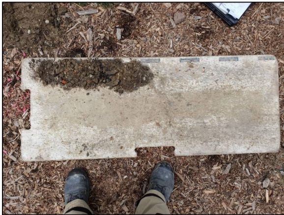
Hand auger met practical refusal at 0.6 m depth on hard material.
