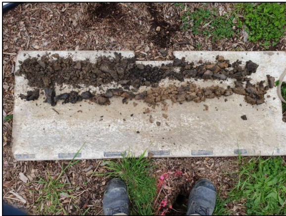
Hand auger met practical refusal at 2 m depth on hard material.
