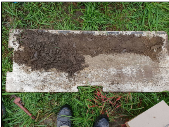
Hand auger met practical refusal at 1.5 m depth on hard material.
