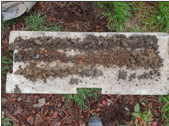
Hand auger met practical refusal at 3 m depth on hard material.
